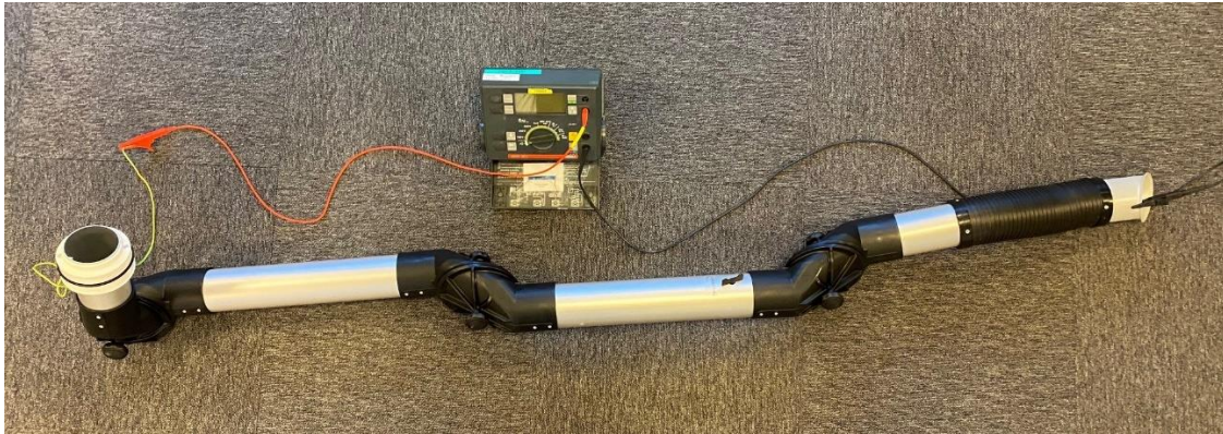
Figure 6: Example: end to end resistance \varnothing 76
